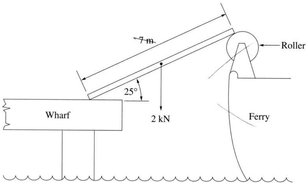
Sketch a free-body diagram of the ramp. Show whether the ramp will slip or remain static for these conditions.
