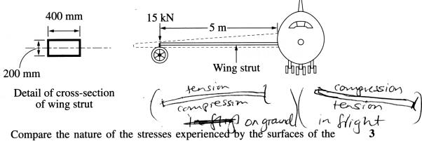
(i) Compare the nature of the stresses experienced by the surfaces of the wing strut when the aircraft is stationary on the ground and when the aircraft is in flight.
