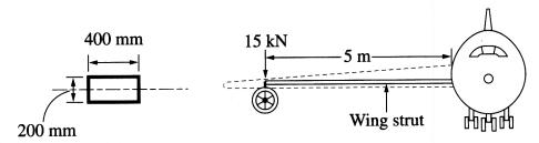
Detail of cross-section of wing strut
