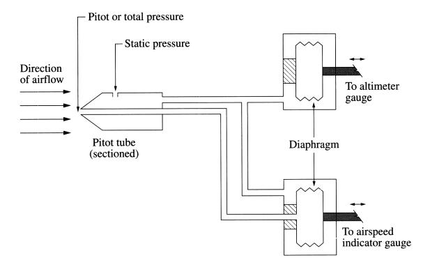
Explain how the airspeed indicator determines airspeed from the pressures sensed by the pitot tube.
