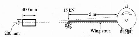
Detail of cross-section of wing strut
