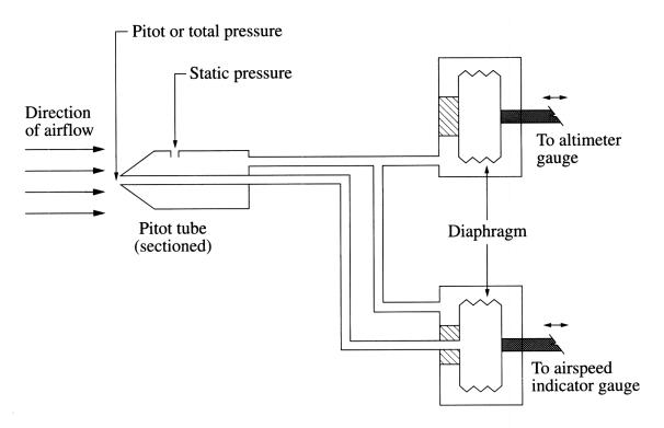
(a) Explain how the airspeed indicator determines airspeed from the pressures sensed by the pitot tube.
