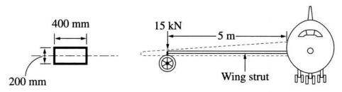
Detail of cross-section of wing strut
