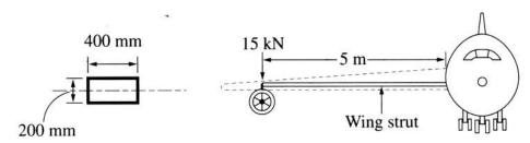
Detail of cross-section of wing strut
