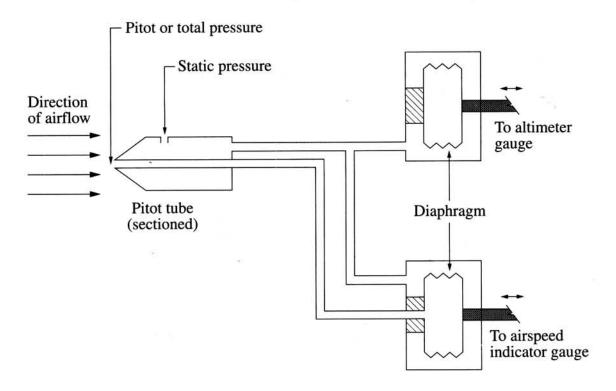
Explain how the airspeed indicator determines airspeed from the pressures
