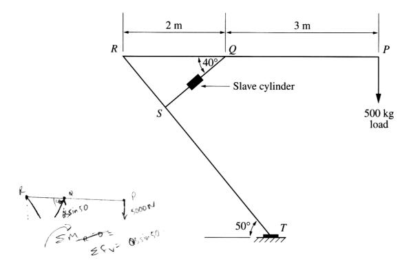
(a) The lifting device is required to hold a load of 500 kg. Determine the minimum force required in member *QS* to keep arm *RP* horizontal.
