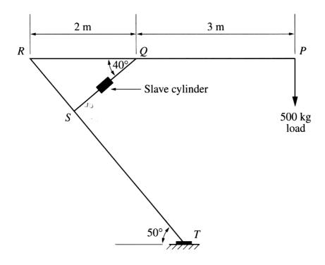
(a) The lifting device is required to hold a load of 500 kg. Determine the minimum force required in member QS to keep arm RP horizontal.
