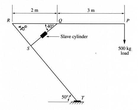
(a) The lifting device is required to hold a load of 500 kg. Determine the minimum force required in member QS to keep arm RP horizontal.
