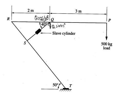
The lifting device is required to hold a load of 500 kg. Determine the minimum (a)
